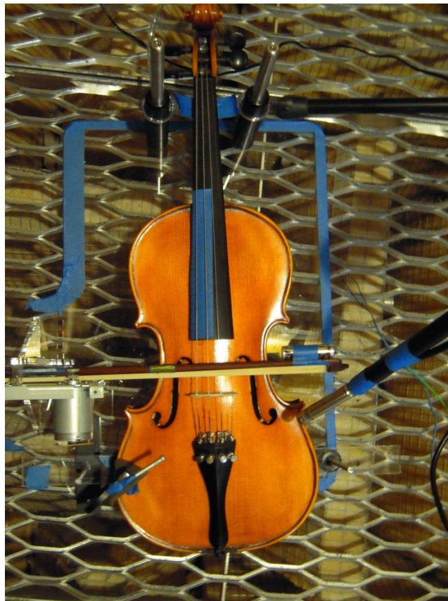
Fig 3. Close-up view of the violin on the bowing machine. The acrylic frame supports the violin at its base and neck, and the corner of the violin is clamped. The bow moves perpendicular to the strings and plays the open-string A note (second string from the left).
