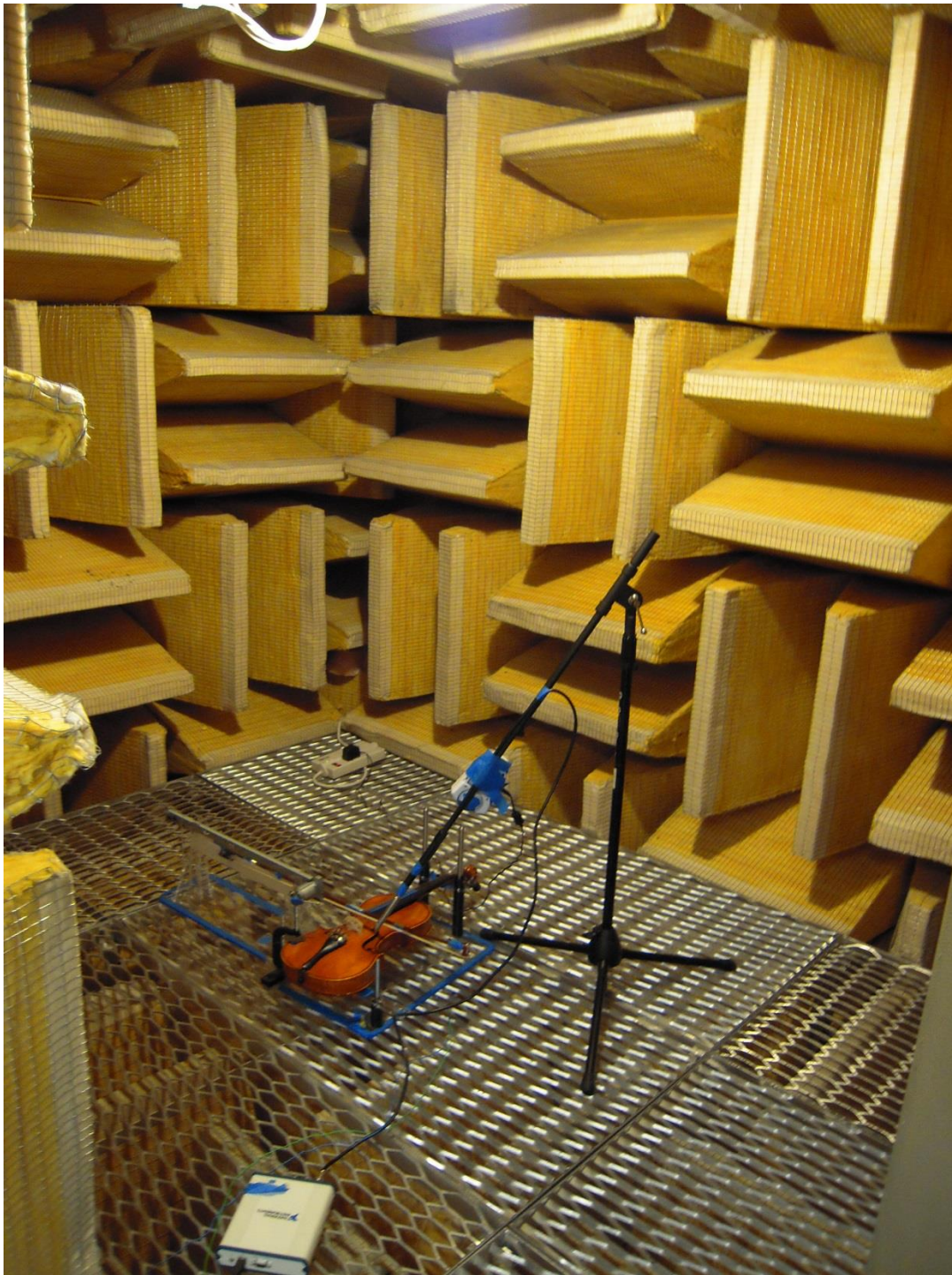
Fig 4. The bowing machine. The setup is controlled from outside the anechoic chamber; flipping a switch causes the belt and the bow to move back and forth. A camera mounted on the microphone stand allows the viewer to watch the tape markings on the bow and record data at the same point every time.
